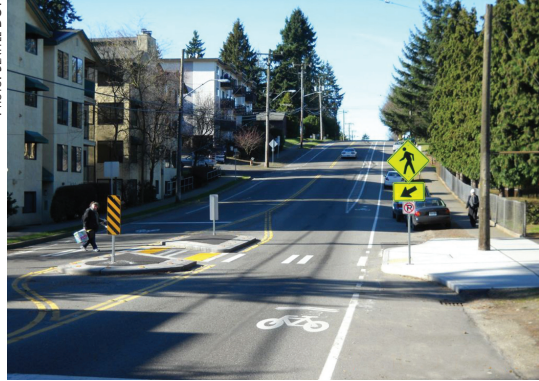
Bicycle lanes, refuge islands, and on-street parking accommodate all users of this Seattle, Washington, street.
